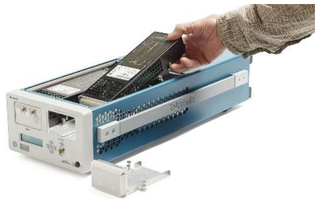
Plugging TSO8C18 module into TSO820 mainframe.
